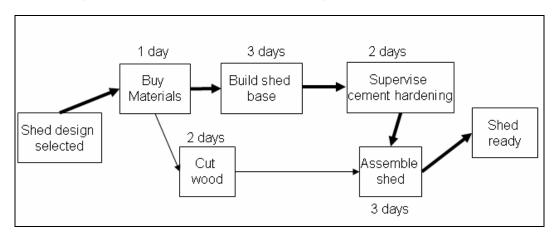
The above network diagram shows the relationships (arrows) between the main activities (rectangles) that are required to build a shed. You can flesh out the following information from the above diagram:
